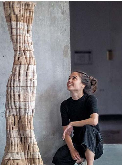
Protomycokion demonstrates the potential of 3D printing with biomaterials in a “new paradigm of manufacturing”: working with nature and biology both as inspiration and as the actual driver of transformation. This Bio-FDM process involves 3D printing with living fungi that bind wood particles after extrusion through their biological growth. In this way, the mycelium grows within the wood composite and fibers it anew while it reaches for nutrients.
